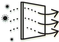
Installation or improvement **FILTERS** in the building's heating and cooling systems (HVAC). Minimum Efficiency Filters (MERV) with a range of 13 or higher can capture 70% of small particles that may contain the infectious virus.
